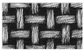
Multifilament Mesh is a woven fabric where each strand consists of many smaller diameter threads, Combines low-cost and disposability
